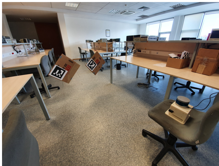
Figure 13: Setting for spatial calibration of stereo camera and LIDAR.
