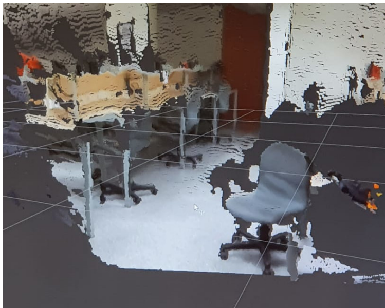
Figure 9: Point cloud data obtained from the stereo camera.
